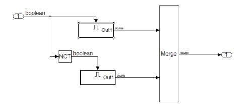
• Enable Action Subsystem inputs from the same If-Else block that provides exclusive execution of the subsystems.
